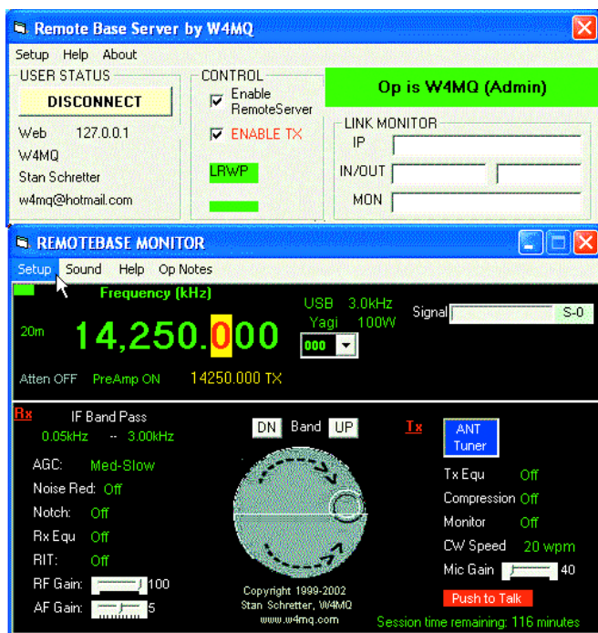
Figure 2—Operation displays used to set up, monitor and control the remote base server.
